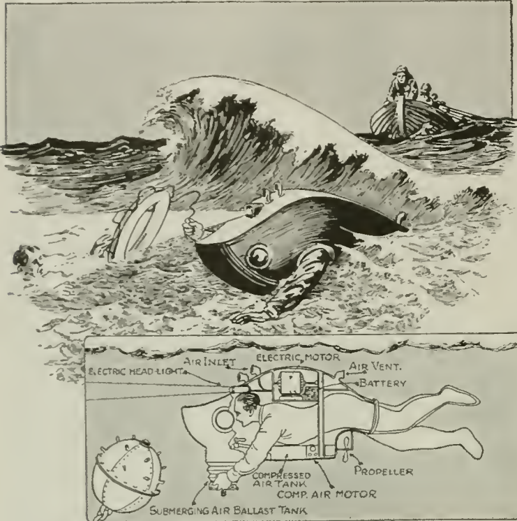
With a Little Ingenuity Amateur Mechanics Can Construct a One-Man Submersible Boat of the Type Here Shown. The Arms and Legs Fit into Flexible Rubber Extensions, the Same as in a Diving Suit. An Electric or Compress Air Motor May Propel the Device.
